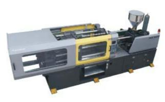
The barrel of **thin wall injection moulding** machine is smaller than it in conventional injection moulding machine. Because the thin wall products need less plastic materials, so if the barrel is as big as the usual one, it will result in the material's dissociation due to the long residence time. And each inject 35%-75% of the maximum injection volume is the best. It should be cautious to choose a thin wall injection moulding machinery company. <u>DAKUMAR</u> is a good choice.
