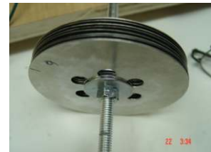
Tesla Turbine can be ran by steam or air
