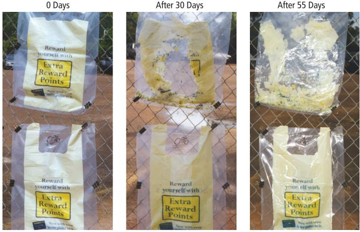
Illustration of photo and thermal degradation of a carrier bag incorporating EPI's TDPA® additive (top row) vs. a bag without EPI's TDPA® additive (bottom row). Test procedures follow ASTM D5272 "Outdoor Exposure Testing of Photo Degradable Plastics" Guidelines.
