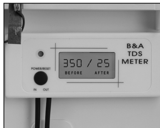
Fig. 14. Water Quality Monitor "ON" Button, Green LED and TDS Readings
