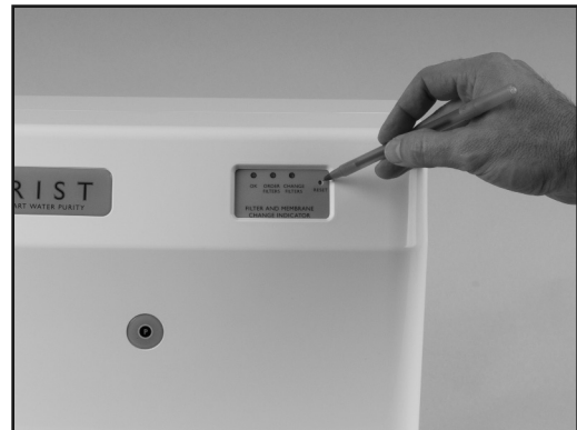
Fig. 24. Awaken the Filter and Membrane Change Indicator
