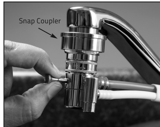
Fig. 13. Pull out Diverter Valve Stem to start cold water flow. Never push in when the faucet is ON.
