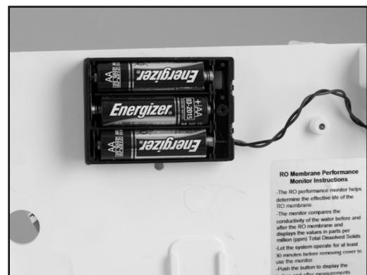
Fig. 22. Use Three AA Batteries
