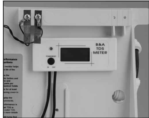
Fig. 9. Water Quality Monitor
